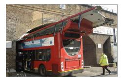
Some arch bridges only allow safe travel for tall vehicles in the centre of the road. You need to read and understand the signs. Failure to do this can be seen in this photo of one of our company's vehicles.
